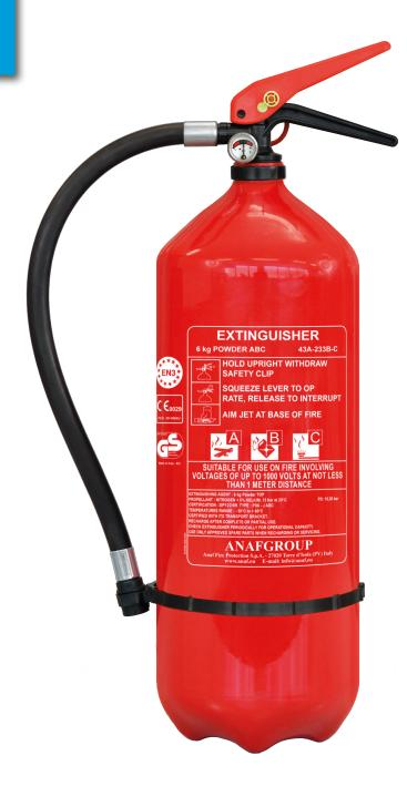
PS6-J TOP is a stored pressure, multi-purpose dry powder fire extinguisher with pressure gauge. Wide operating temperature range -30 °C +60 °C, ensuring suitability for use in low-temperature countries. Certified to the Pressure Equipment Directive PED 2014/68/EU, to the Marine Equipment Directive MED 2014/90/EU and CEN EN3-7. 100% of the fire extinguishers are checked by an electronic helium leak detection system.
